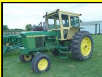
JD 4020 Dsl, Cab, Side Console, 8478 Hrs Showing, 3pt, 2 Hyds, New 18.4-38's, 10.00-16 fronts, New Style Step, Front Weights, SN # 255090R
